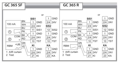
► Connect the sensor to the power supply.
