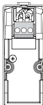
Break to the cable duct opening.
